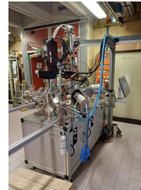
The UHV system for X ray photoemission @LHe T.
