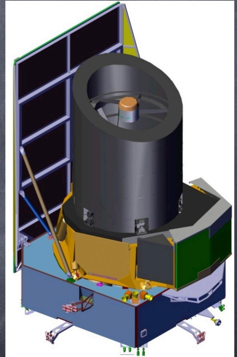
Observed with a **mini** structure: mirror ~1.2 m  $\varnothing$
