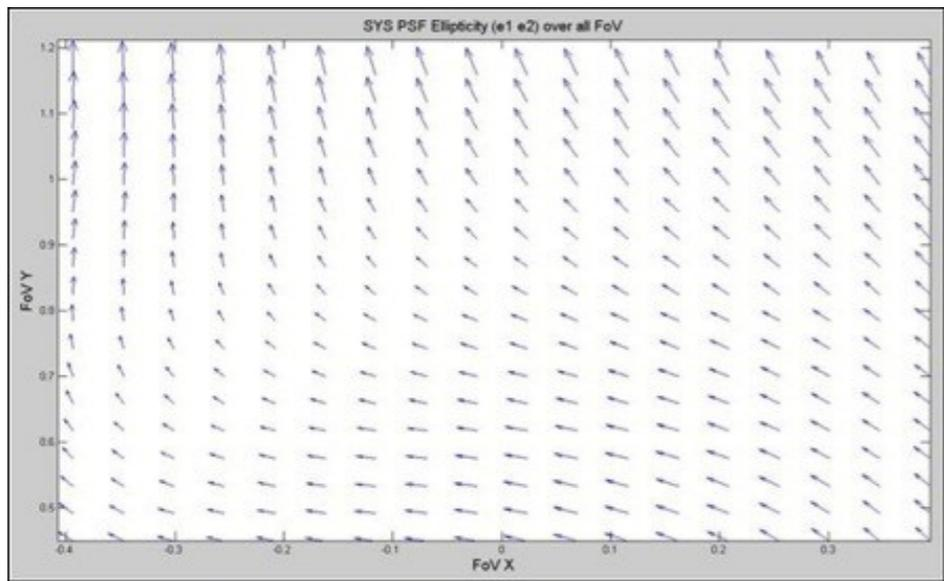
Figure 38: Euclid system VIS PSF ellipticity vector ( $e_1, e_2$ ) map over the reference system full FoV
