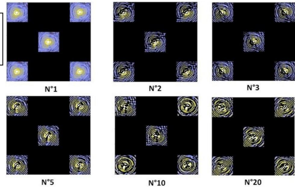
Figure 39: VIS PSF eigenvectors and residuals as a function of number of eigenvectors used in the reconstruction of a given Euclid PSF
