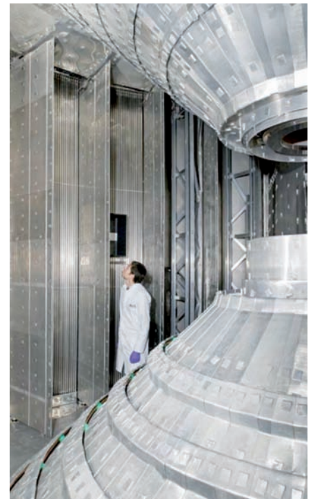
Figure 5. The inside of the LET detector tank. The whole tank is lined with Cadmium. Detectors are 4 m high and are in packs of 32 tubes separated by vertical vanes.
